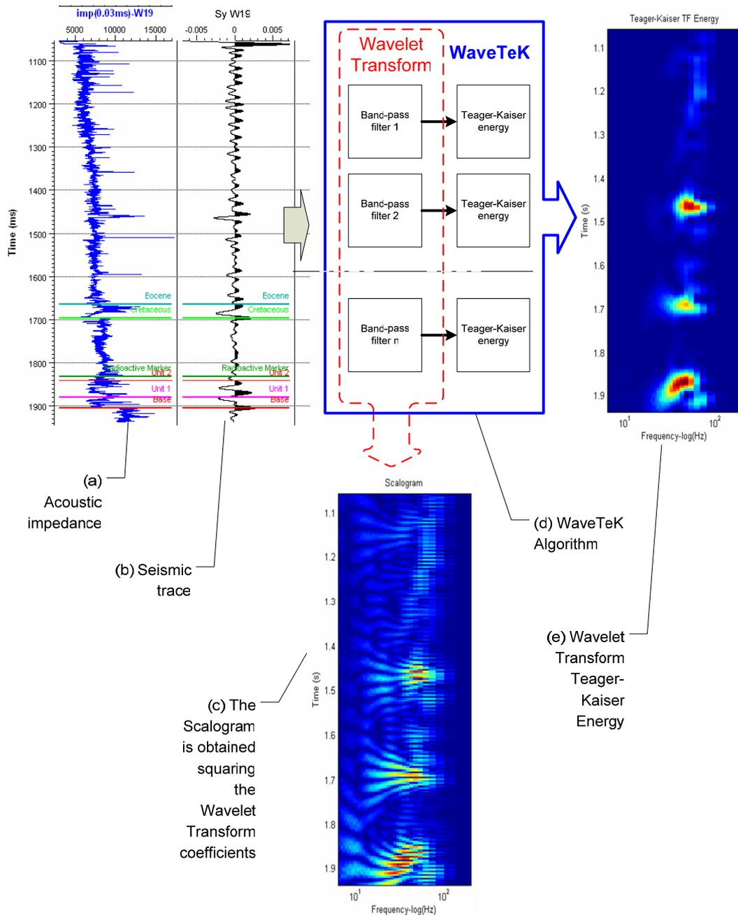
Figure 1: The WaveTeKE algorithm: a) Acoustic impedance; b) Synthetic seismic trace; c) The wavelet transform scalogram; d) WT as a filter bank followed by the Teager-Kaiser Energy estimator; e) The WaveTeKE result.
