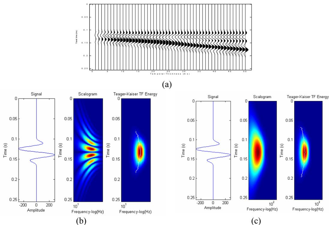
Figure 2: a) Filtered wedge model; b) The seismic trace with 10 ms temporal thickness, the WT scalogram obtained using the real Morlet wavelet and the WaveTeK; c) The seismic trace with 10 ms temporal thickness, the WT scalogram obtained using the complex Morlet wavelet and the WaveTeK.
