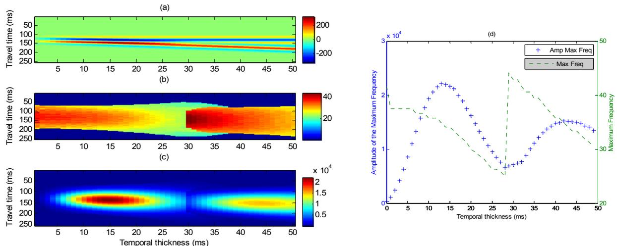
Figure 3: a) Filtered wedge model; b) The maximum instantaneous frequency versus temporal thickness; c) The amplitude of the maximum instantaneous frequency obtained through the ridge WaveTeK versus temporal thickness; d) Time interval seismic attributes: the Maximum Instantaneous frequency and the associated maximum amplitude versus temporal thickness.
