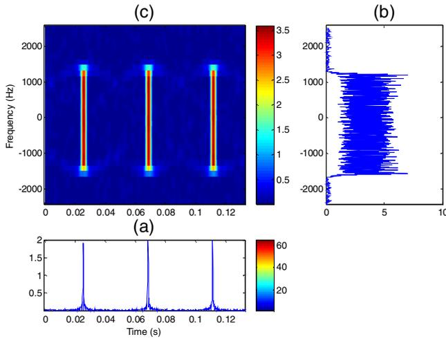
Figure 1 – Classic model for helicopter echo: (a) signal in time domain; (b) FFT spectrum of the signal; (c) STFT spectrogram
