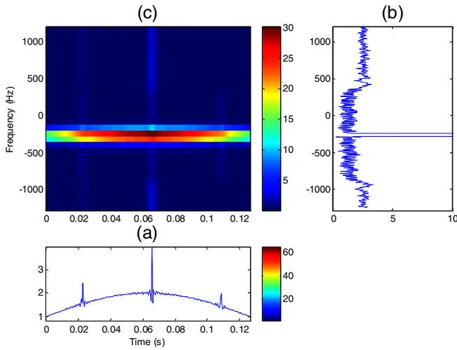
Figure 3 – Undersampled helicopter echo: (a) signal in time domain; (b) FFT spectrum of the signal; (c) STFT spectrogram
