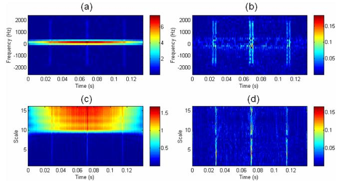
Figure 8 – Effect of finite differentiation in STFT and CWT: (a) STFT spectrogram of the signal; (b) finite differentiation of the STFT; (c) CWT of the signal; (d) finite differentiation of the CWT
