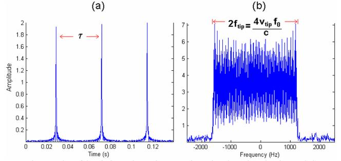
Figure 4 – Obtaining the L/N quotient in the classical model: (a) time between peaks; (b) blade tip velocity
