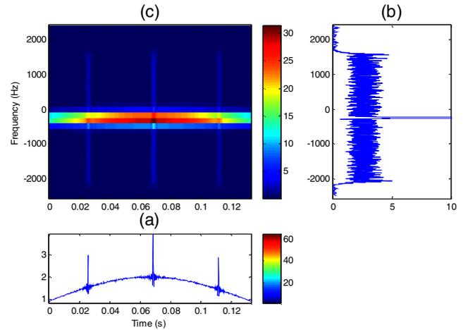
Figure 2 – Helicopter echo with fuselage component: (a) signal in time domain; (b) FFT spectrum of the signal; (c) STFT spectrogram
