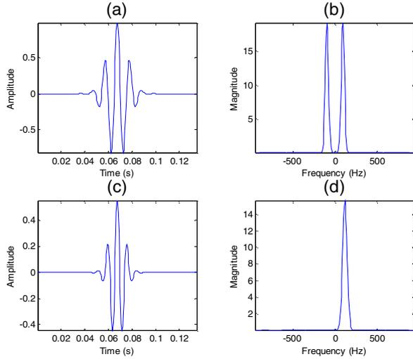
Figure 5 – Morlet Wavelet: (a) real part of the Real Morlet Wavelet in time domain; (b) absolute value of the Real Morlet Wavelet in frequency domain; (c) real part of the Complex Morlet Wavelet in time domain; (d) absolute value of the Complex Morlet Wavelet in frequency domain;
