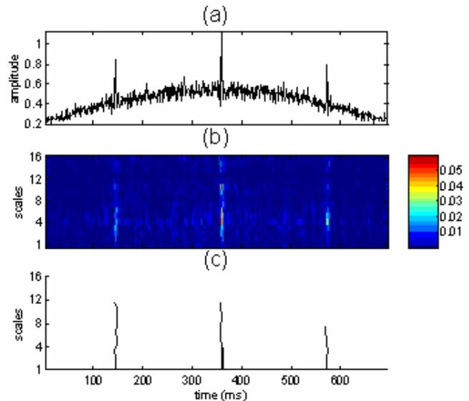
Figure 10 – (a) Signal in time domain; (b) Teager-Kaiser energy of the CWT after finite differentiation; (c) Wavelet transform modulus maxima lines (WTMML).
