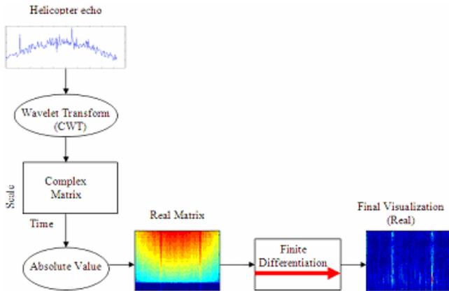
Figure 7 – Finite differentiation of the CWT
