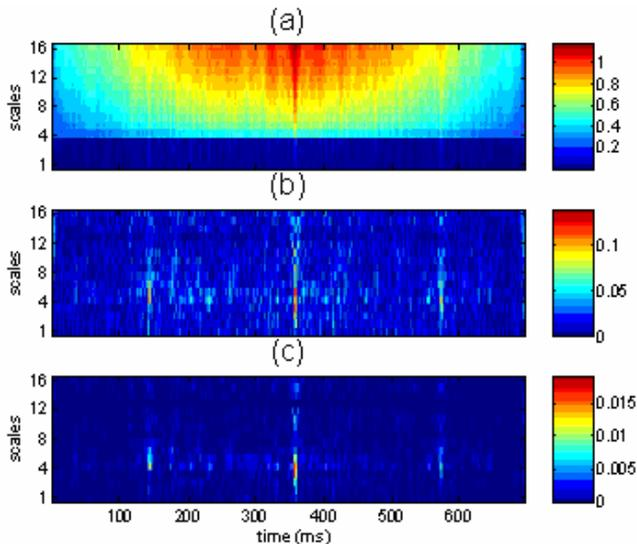
Figure 9 – (a) CWT of the signal; (b) CWT of the signal after finite differentiation; (c) Teager-Kaiser energy of the CWT after finite differentiation
