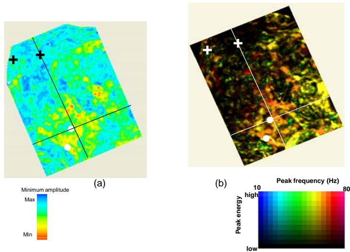
Figure 5: 80-ms time interval seismic attributes: (a) Minimum amplitude and (b)  $\max_{f,t} E(f,t)$  given by equation 2. White circles represent producer well locations. Crosses represent non-producer well locations.
