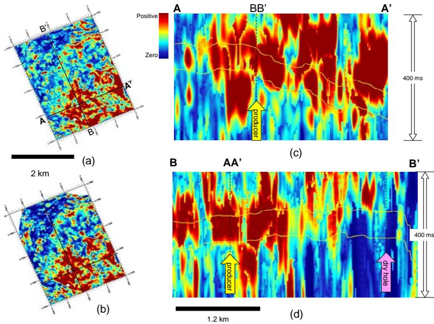
Figure 4: (a) Horizon slice through the TE energy volume.(b) Formation attribute map of the TE absolute sum value between the top Horizon and 80 ms below WaveTeKE instantaneous amplitude along (c) line AA' and (d) line BB'.
